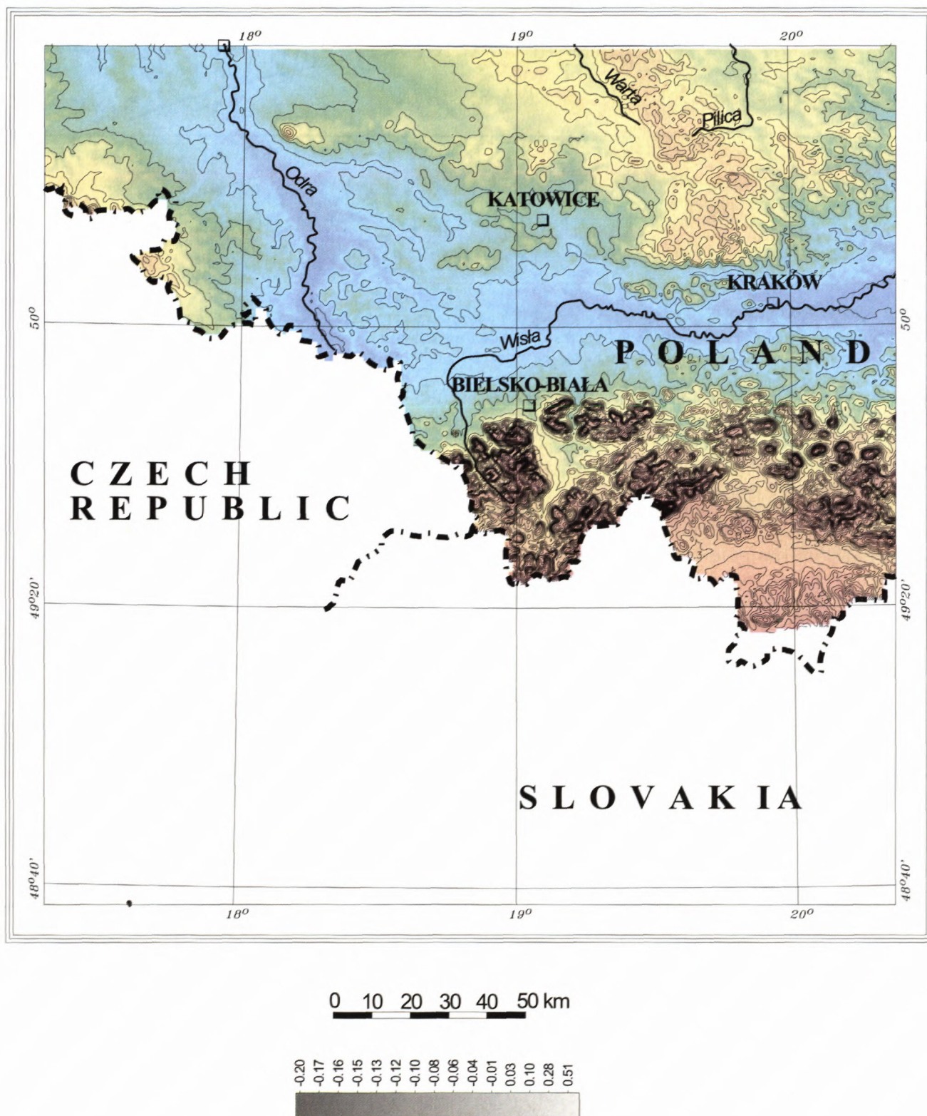
Fig. 2 Terrain correction map for the whole area in external zone (22.5 166.7km)
